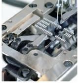
If the looper thread is pulled at the end of sewing, this thread trimmer prevents unraveling with STITCHLOCK. Use of this thread trimmer eliminates the need for a bartacker. In addition, there is no need to perform manual thread trimming using scissors. As a result, the quality of sewn products and operational efficiency is dramatically increased.
