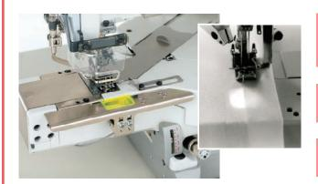
This attachment illuminates the bottom fabric from below, so the operator can perform hemming operations while checking the edge of the folded fabric. Thanks to this feature, hemming is as easy as plain seaming. Deskilling the operation and increasing efficiency achieves high quality products.
