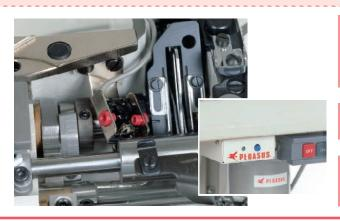
If the looper thread is broken during sewing, the sensor detects this malfunction and the machine automatically stops. This device reduces trouble caused by looper thread breakage and decreases the time and labor required for troubleshooting. All subclasses can use this device.
