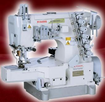
2 or 3 needle, flatbed, interlock stitch machine 2 or 3 needle, cylinder bed, interlock stitch machine
