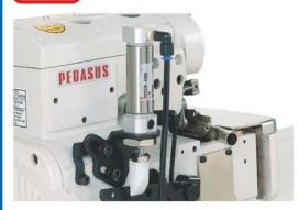
Pressing the treadle with your heel raises the presser foot. This device is easy to use, thus decreasing operator fatigue and increasing productivity.
