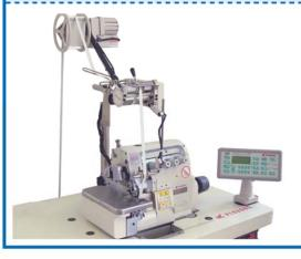
The tension-adjustment type elastic feeder (MU) feeds the elastic lace according to preset data while adjusting tension exerted on the elastic lace, so uniformly finished and quality products are obtained.
